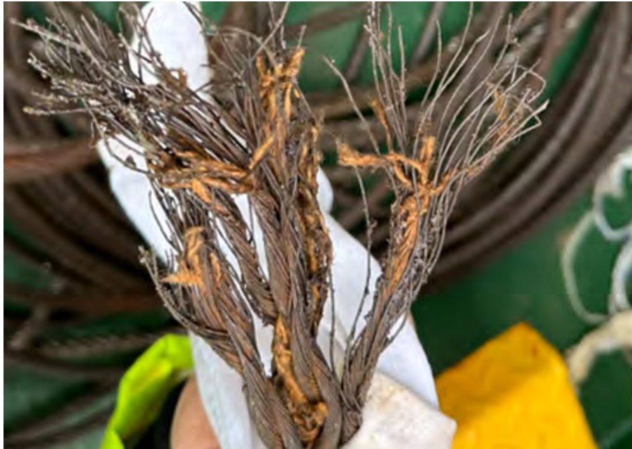
Figure 21: Wire rope breakage.
